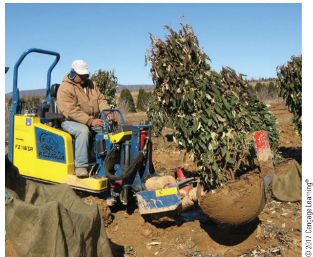
▲ Figure 1-4 Nursery equipment operator digging a deciduous tree with a Pizzaglia vibratory digger.
